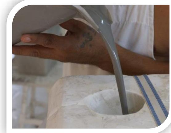
filling process, in the mold
